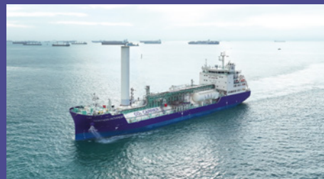
液化CO 2 輸送船 NORTHERN PIONEER (提供: Northern Lights JV DA)
