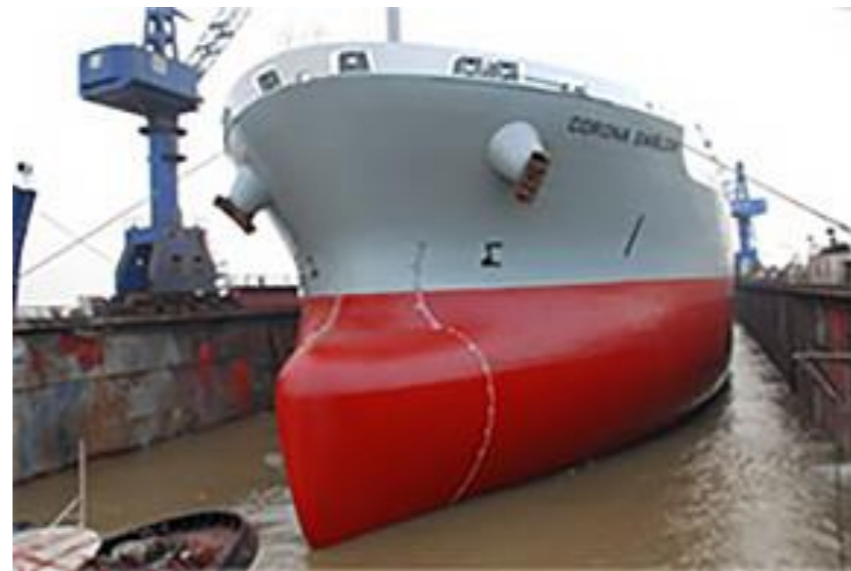
A ship being coated with silicone paint (red color) at the Dry dock
