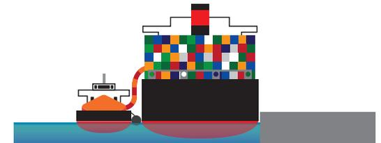
A method of bunkering where an LNG bunkering vessel comes alongside an LNG-fueled vessel to supply LNG at different locations such as along the quayside, pier or at anchor.
