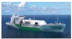
LNG Bunkering Vessel (illustration courtesy of Kawasaki Heavy Industries)
