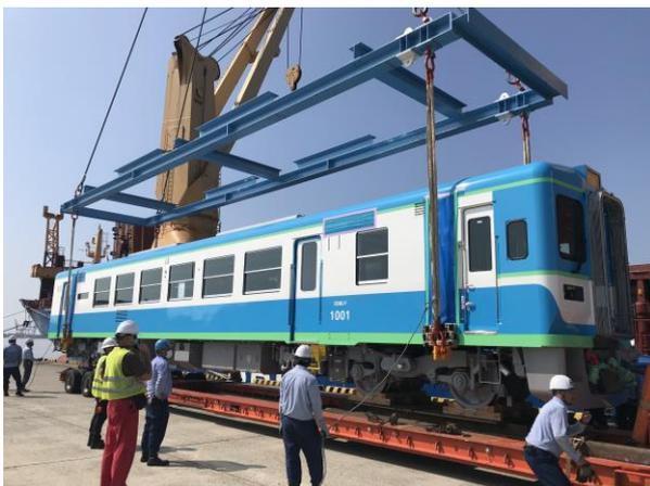
Cargo operation using ship’s crane
