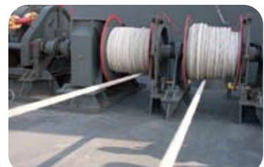
① **Mooring winch:** Equipment that reels in rope and wire used in mooring the ship to berth.
