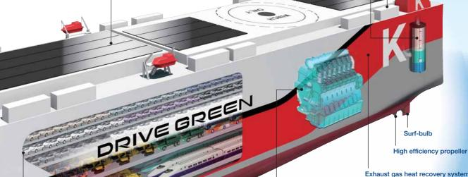
Exhaust gas heat recovery system for diesel generator (exhaust gas economizer for diesel generator)
