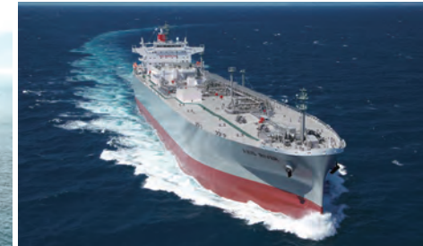
LPG and Ammonia Carrier AXIS RIVER
