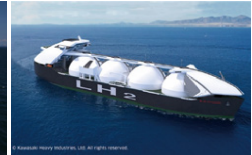
Concept image of 160,000 m³ scale liquefied hydrogen carrier (Image provided by Kawasaki Heavy Industries, Ltd.)
