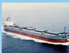
The wide-beam / shallow draft coal carrier *CORONA ACE*, the basic type for the transportation of thermal coal, was completed.
