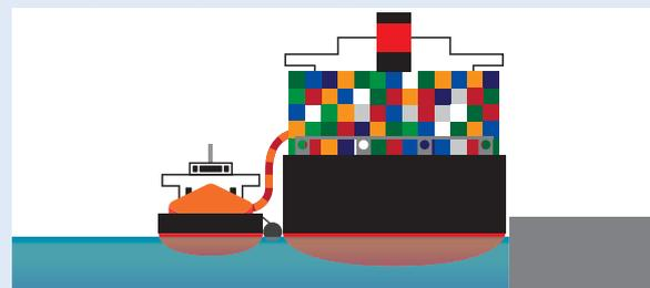
A method of bunkering where an LNG bunkering vessel comes alongside an LNG-fueled vessel to supply LNG at different locations such as along the quayside, pier or at anchor. (From left to right : LNG bunkering vessel, LNG-fueled vessel)
