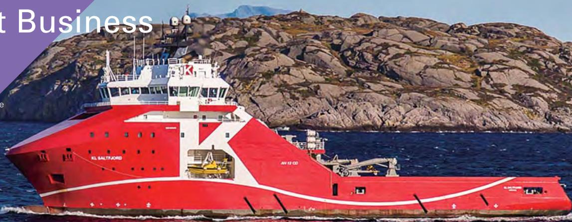
Anchor Handling Tug Supply (AHTS) Vessel
