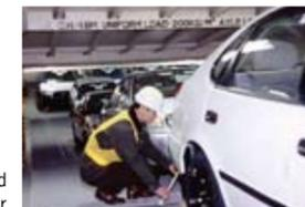
Inspecting whether a vehicle is secured properly on a car carrier
