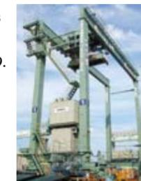
Compared to conventional models, the hybrid cranes consume less fuel and produce less carbon dioxide. In addition, improved engines generate much less noise.
