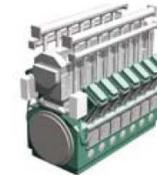
Two sets of gas engines (5,000kw each) are applied as propulsion system, employing lean burn combustion. Each cylinder has an auxiliary chamber with spark plug to generate a flame for ignition, which is called torch jet, with the air-gas fuel mixture being combusted in the main chamber.
