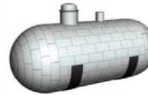
Two pressure vessels (type C, 6 bar) are applied for LNG fuel tanks. These tanks shall be required to comply with strict safety standards. Therefore, the tanks are installed in an independent compartment and located a certain distance from the ship's outer shell and bottom to ensure safety in the event of a collision or other marine incident. In addition, a complete double-wall piping system is applied for fuel pipes as a further safety measure.
