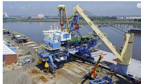
Shiploader: Port facilities used for loading dry bulk cargo as Iron ore
