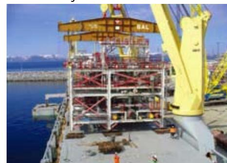
Project cargo : Assembled modules of LNG plant
