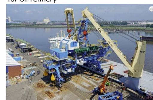
Shiploader: Port facilities used for loading dry bulk cargo as Iron ore
