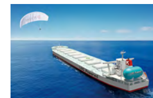
LNG-fueled Capesize Bulk Carrier and Seawing
