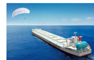
LNG-fueled Capesize Bulk Carrier and Seawing
