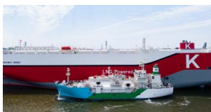
LNG bunkering vessel, KAGUYA, and LNG-fueled car carrier CENTURY HIGHWAY GREEN (Image provided by Central LNG Marine Fuel Japan Corporation)
