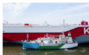
LNG bunkering vessel, KAGUYA, and LNG-fueled car carrier CENTURY HIGHWAY GREEN (Image provided by Central LNG Marine Fuel Japan Corporation)
