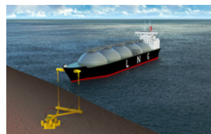
Image of FSRU mooring (Image provided by SOFEC, Inc.)
