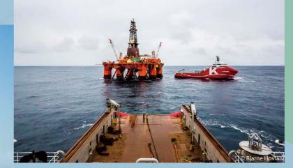
Anchor handling tug supply vessel performing a rig move Photo: Bjarne P. Hovland
