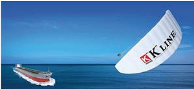
The kite, which is installed on the bow of the vessel, is operated and deployed from the bridge.
