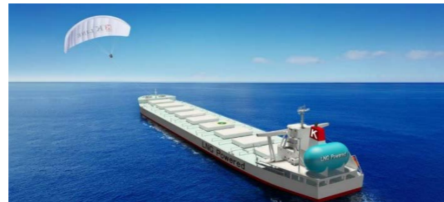
It assists the propulsion power of the vessel by utilizing wind power under fixed conditions for wind strength and direction.
