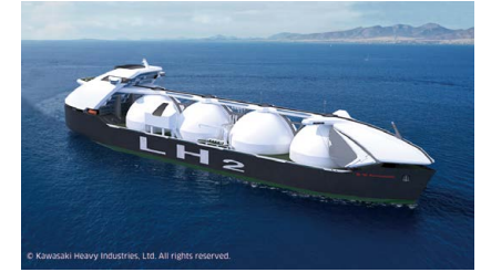
Concept image of a 160,000 m 3 liquefied hydrogen carrier provided by Kawasaki Heavy Industries, Ltd.
