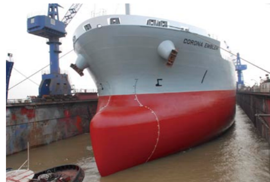
A ship being coated with silicone paint (the red colored part) at the dry dock.
