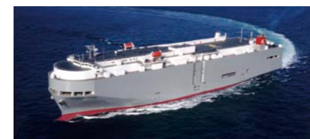
Heat shield paint is highly effective for a car carrier because the accommodations and upper part of the bridge are wide.
