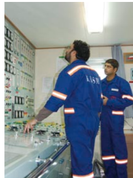
Cargo oil discharging rate being controlled at a tanker
