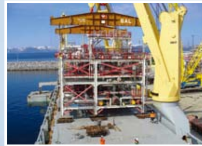
Project cargo: An assembled module for an LNG production facility
