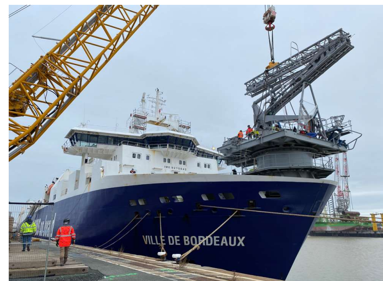
Installing Seawing's machinery part to trial vessel
