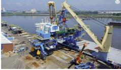
Shiploader : Port facilities used for loading dry bulk cargo as Iron ore
