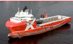
●Platform Supply Vessel (PSV) PSVs are "sea trucks" used mainly to transport materials and fuel to offshore rigs. The company's new PSVs, with length 95 meter and width 20 meter, are among the world's largest, with deadweight capacity of 5,100 tons and deck area of 1,100 square meters. Those vessels also have latest equipment and systems such as DPS.
