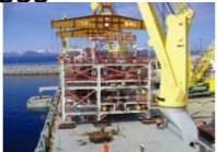
Project cargo: Assembled module of LNG plant
