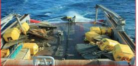
•Anchor Handling Tug Supply(AHTS) vessels AHTSs engage in support activities when offshore drilling rigs are moved from location to location, such as raising anchors from the seabed, rig towing. AHTS also engages in support activities for seabed pipeline laying works.
