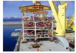
Project cargo: Assembled modules of LNG plant
