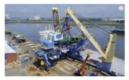
Shiploader: Port facilities used for loading dry bulk cargo as Iron ore
