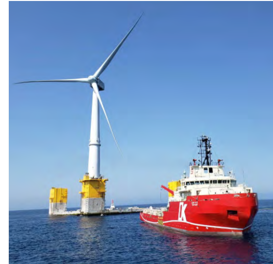
Image courtesy of KAWASAKI KINKAI KISEN KAISHA, LTD. Akatsuki Offshore Support Vessel towing a floating off-shore wind turbine
