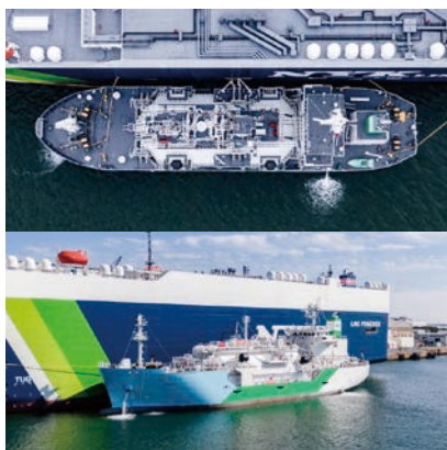
Kaguya supplying LNG fuel with ship-to-ship bunkering basis (photo provided by Central LNG Marine Fuel Japan Corporation)
