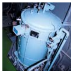
Oily water Separator
