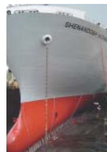
SHENANDOAH HIGHWAY, to which silicon paint is applied
